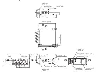
SUSPENSION BOLT: W3/8(M10) REFRIGERANT PIPE FLARED CONNECTION
