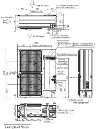
1 ·· Refrigerant GAS pipe connection (FLARE) ø15.88 (5/8F) 2 ·· Refrigerant LIQUID pipe connection (FLARE) ø9.52 (3/8F) \*1 ·· Indication of STOP VALVE connection location.
