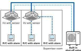
\* Solid lines are refrigerant piping. Dotted lines are communication lines
