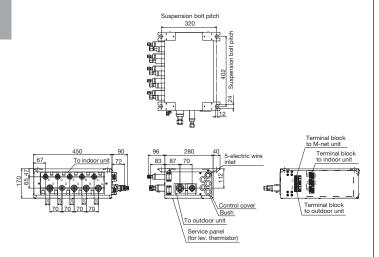
Suspension bolt : W3/8(M10) Refrigerant pipe flared connection
