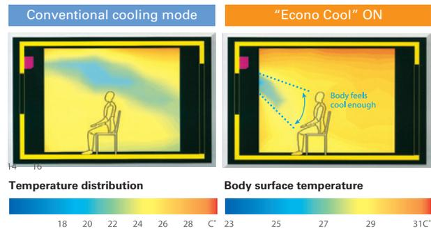
Ensures more comfort even when the set temperature is 2°C higher than the conventional cooling mode.
