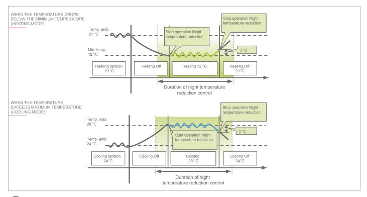
If the room temperature is measured at the intake of the indoor unit, the temperature cannot be accurate when the indoor unit is stationary. In this case, provide a remote sensor (PAC-SE41TS-E) or move the temperature acquisition using the integrated sensor to the remote control.
