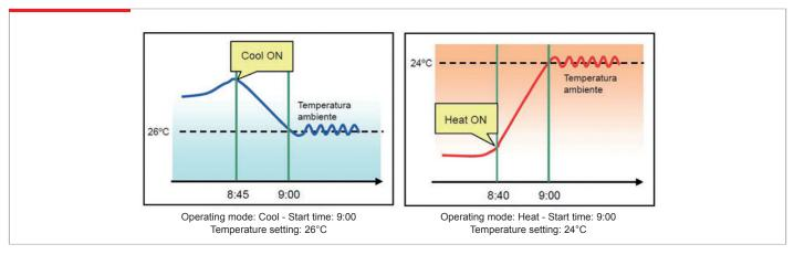
The 'Optimised Start' and 'Night Setback' (or 'Maintenance Temperature') functions are perfectly integrated and complement each other. Having the room at a maintenance temperature and anticipating the switch-on time with respect to the time schedule ensures maximum comfort for the occupants exactly when required by the time schedule.
