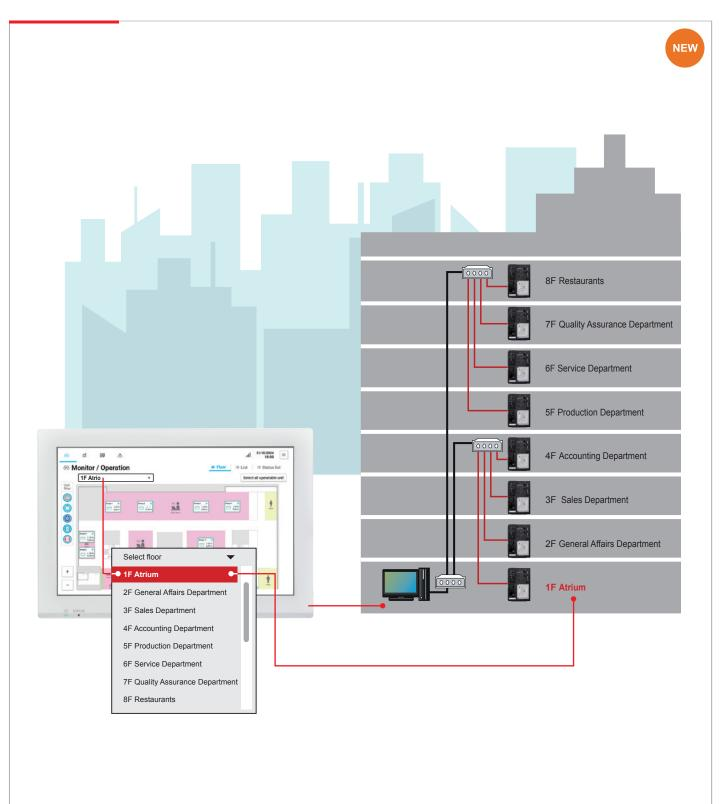
Connection function to the centralised BACnet monitoring system®
