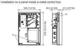
(A) Installation frame (supplied part D-12) (B) Controller mounting hole
