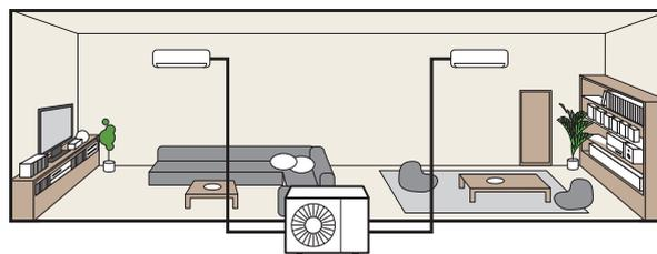
**Attention** MXZ-DM is exclusively for connection to MSZ-HJ and DM. Please check to make sure that wiring is done correctly.
