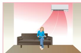
If the heating operation is continued, the warm air is formed around ceiling.
