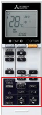
The remote controller is equipped with buttons that are used exclusively for setting the Weekly Timer. Setting operation patterns is easy and quick.
