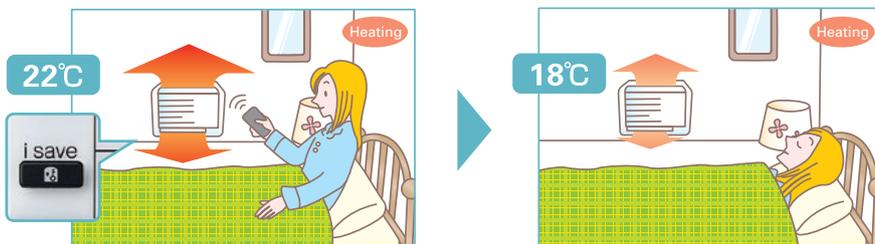
\* Temperature can be preset to 10°C when heating in the "i-save" mode.
