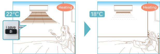
\* Temperature can be preset to 10°C when heating in the "i-save" mode.
