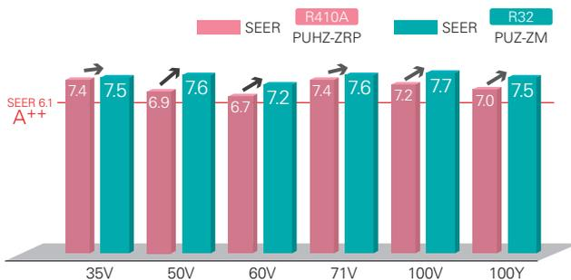
Introduction of new R32 refrigerant reduces energy consumption and realises energy savings.
