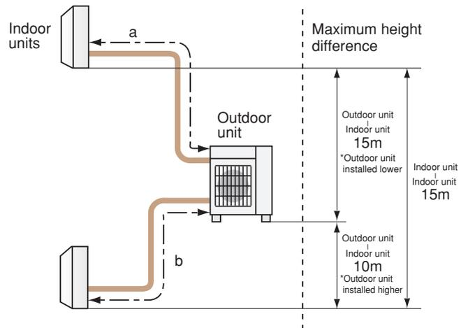
\* When connecting MFZ-KJ Series indoor unit to MXZ-2D42VA2 or MXZ-2D53VA(H)2, additional refrigerant is required. For details, please contact Mitsubishi Electric.
