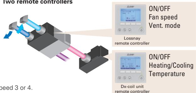
When using only one remote controller, Lossnay fan speed is fixed at fan speed 3 or 4.
