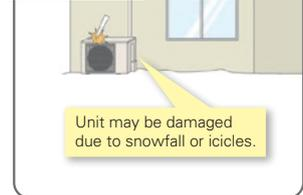
Use a stand to add sufficient height to protect the unit heat exchanger from snow and prevent icicles forming during defrost operation.
