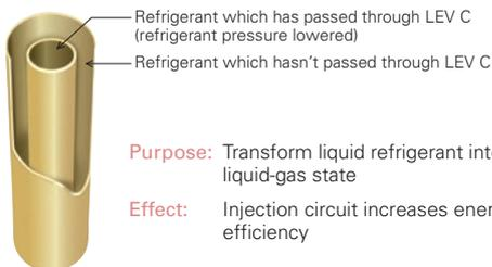
The compressor is subjected to a heavy load when compressing liquid refrigerant, and the result is lower operation efficiency. The addition of HIC supports refrigerant heat exchange at two different pressure levels. The heat-exchange process transforms the injected liquid refrigerant into a gas liquid state, thereby decreasing the load on the compressor during the compression process.
