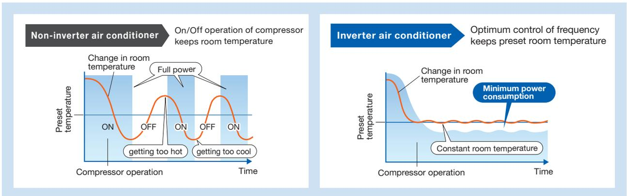
The compressors of air conditioners without an inverter start and stop repeatedly in order to maintain the preset room temperature. This repetitive on/off operation uses excessive electricity and compromises room comfort. The compressors of air conditioners equipped with an inverter run continuously; the inverter quickly optimizing the operating frequency according to changes in room temperature. This ensures energy-efficient operation and a more comfortable room.
