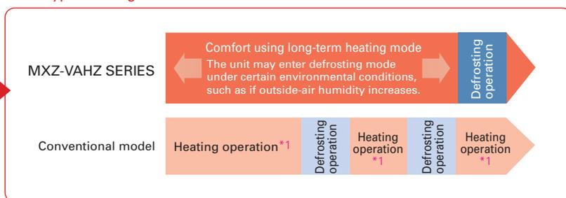
\*1: Conventional model performs continuous heating approximately 30min up to a maximum of 90min.
