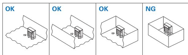
If you unavoidably install a unit in a space where all four sides are blocked or there are depressions, confirm that one of these situations (A, B or C) is satisfied.
