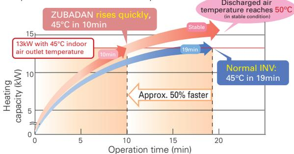
■ Operation at  $-20^{\circ}\text{C}$  outdoor temperature
