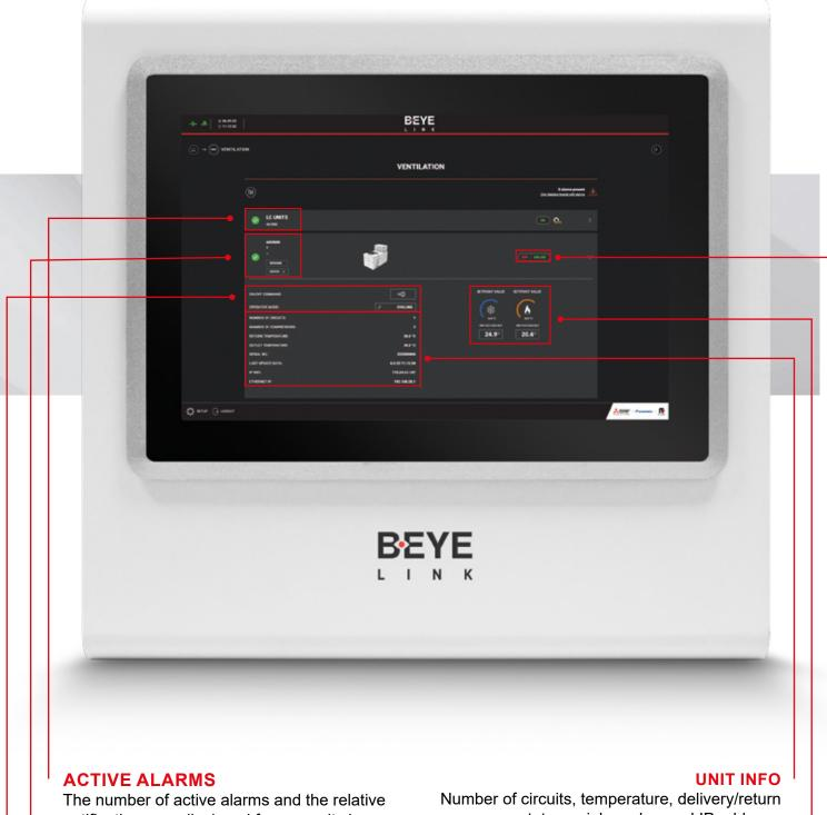
notifications are displayed for any units in an alarm state. More details are available by accessing the web server page for the units (KIPLink).
