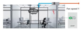
■ Automatic operation with CO<sub>2</sub> sensor and PZ-62DR-E Fan speed automatically changes depending on CO<sub>2</sub> concentration.
