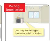
Use a stand to add sufficient height to protect the unit heat exchanger from snow and prevent icicles forming during defrost operation.
