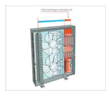
coil itself against corrosion, ensuring that the unit continues to function with the same outstanding thermal exchange efficiency and performance over time
