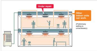
Reduction in the stoppage time of the heating operation prevents drops in room temperature.
