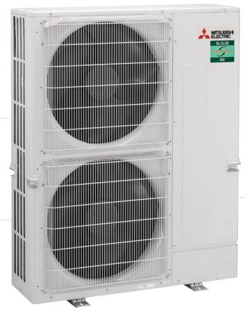
OUTDOOR UNIT THAT BENEFIT FROM SCROLL COMPRESSOR, IS ALSO EQUIPPED WITH A DEVICE CALLED "POWER RECEIVER", A REFRIGERANT ACCUMULATOR ACCOMPAINED BY A PAIR OF LEV VALVES, WITH THE DUAL FUNCTION (SUBCOOLING/OVERHEATING THE REFRIGERANT).
