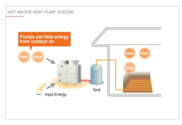
The lower outdoor temperature limit for  $70^{\circ}\text{C}$  hot water output has been extended from -10°C in the conventional model to -20°C in the new model. The operating temperature range has also been improved from "-20°C to 40°C" to "-25°C to 43°C". It is suitable for heating and heat-retention operations.
