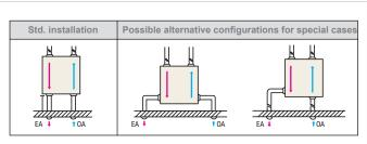
\*Changing the installation configuration causes no any additional pressure loss.
