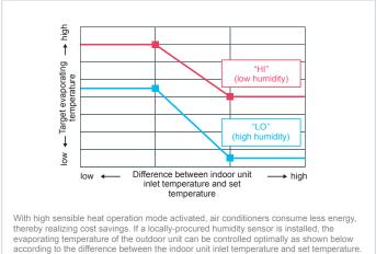
according to the difference between the indoor unit inlet temperature and set temperature. A wide range of temperature settings are available, from a low evaporating temperature close to the temperature for normal operation to a high evaporating temperature to realize energy savings.
